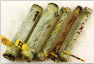
Competitor lubricant (significant corrosion)
